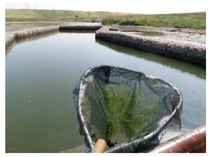
This second photo shows the results of a double deep sweep (approx. 2 m) along the inside of the wall approximately 10 m from the inlet on the east side (photo is facing south). The organics collected in the screened material include short filaments of algae and freshwater shrimp.
