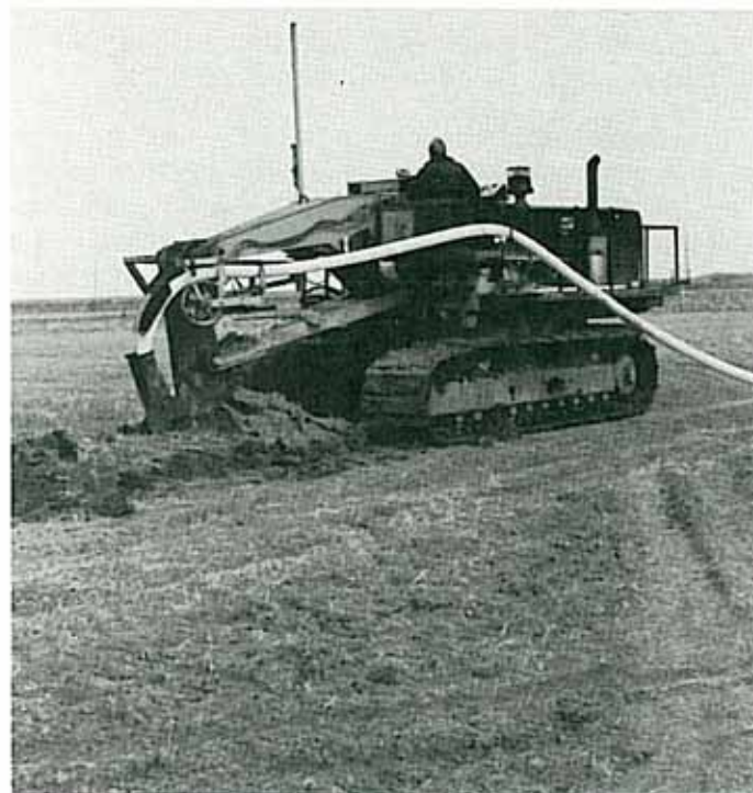
The Canadian built Wolfe plow is installing up to 8200 lineal metres of tubing a day.
