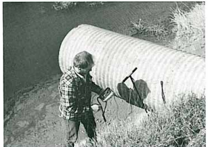
On site tests included soil and water resistivity, soil and water pH, and soil to pipe electropotential.
