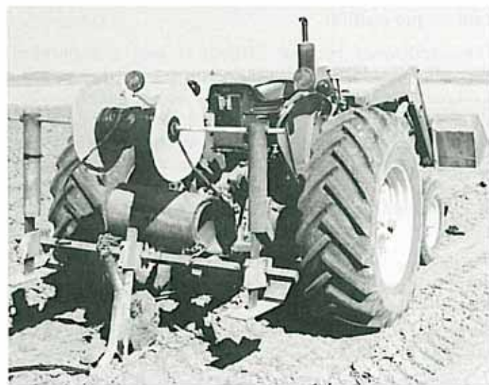
The typhoon dripper line is installed into the soil by the plough method.
