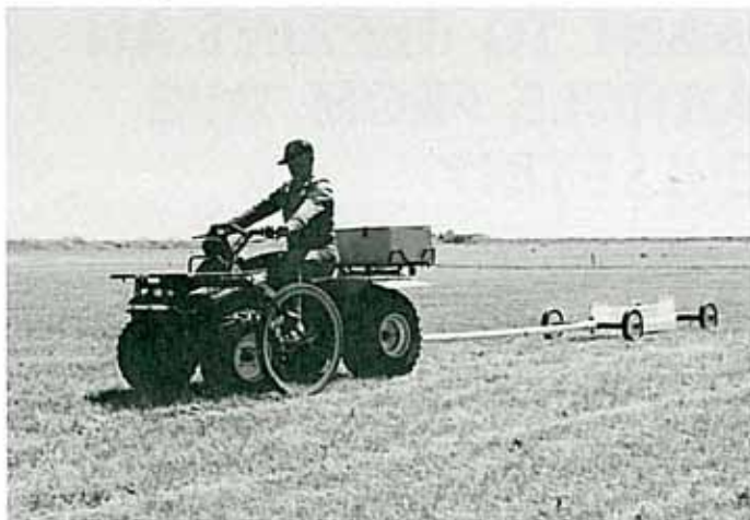
Automated EM-38 salinity mapping system.
