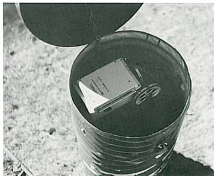
Alberta Agriculture has discontinued use of corrugated metal pipe and steel recording wells to house their electronic dataloggers.
