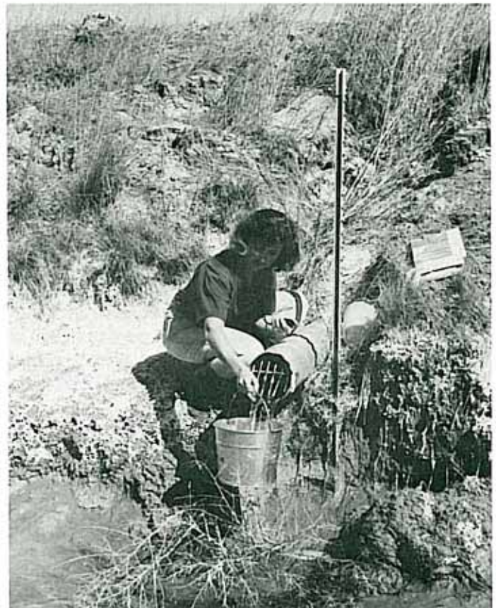
Technologist Bonnie Hofer takes flow measurement and sample for water quality analysis.
