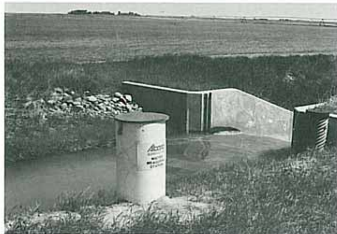
Typical Alberta Agriculture PVC recording well.
