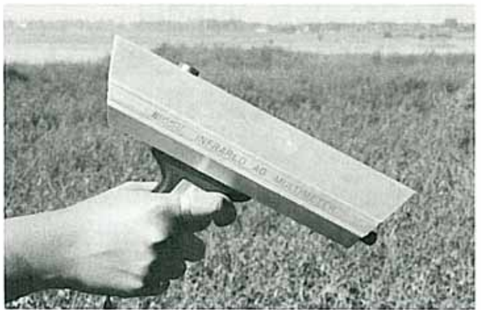
Hand-held infrared gun obtaining crop canopy temperature.
