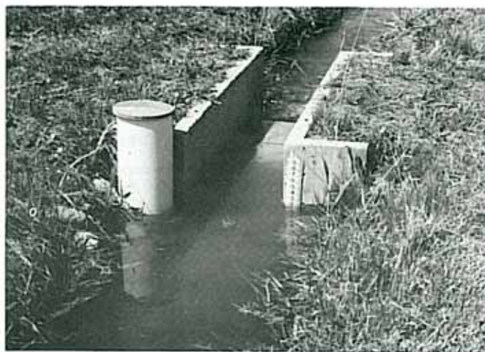
The Broad-Crested Weir received the highest rating of the five tested.
