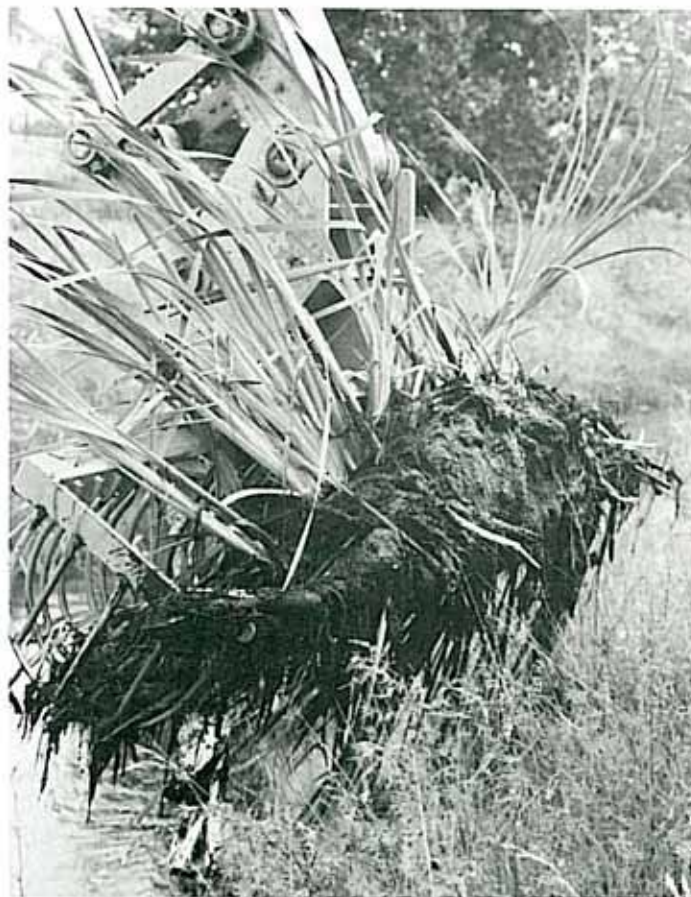
Basket removes cattails including root material.
