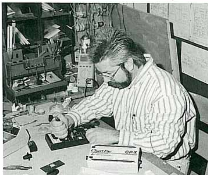
Technologist Don Roth replaces integrated circuit chip in electronic datalogger.
