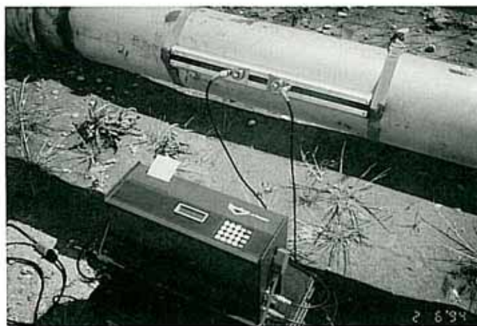
Ultrasonic flow meter is easily clamped onto a pipeline (no drilling required).
