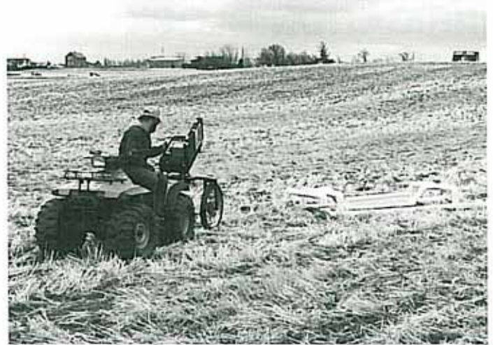
EM-38 electromagnetic conductivity meter being pulled across field measuring soil salinity.
