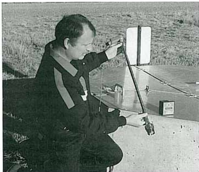
Steve Topping holds Seaflow meter that needs only 12-volt marine battery to power it.
