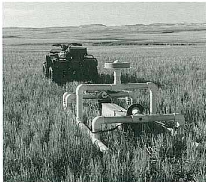
GPS unit sits on top of sled being pulled by ATV.
