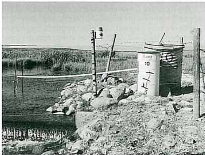
Crowfoot Creek Site 10, showing tipping bucket rain gauge, stilling well enclosure, ISCO sampler enclosure, and ISCO sample intake line.
