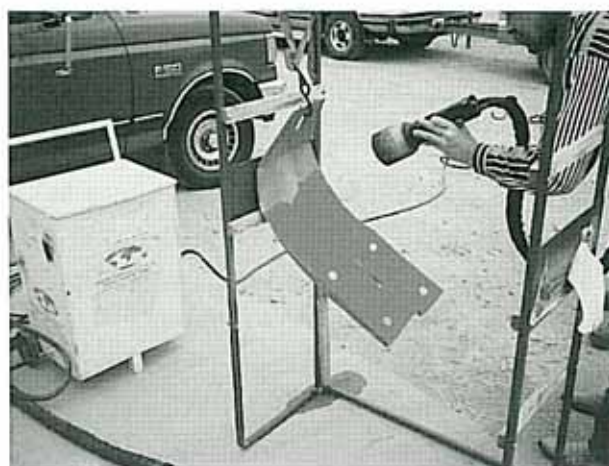
Thermoplastic coating being sprayed on sheet metal.
