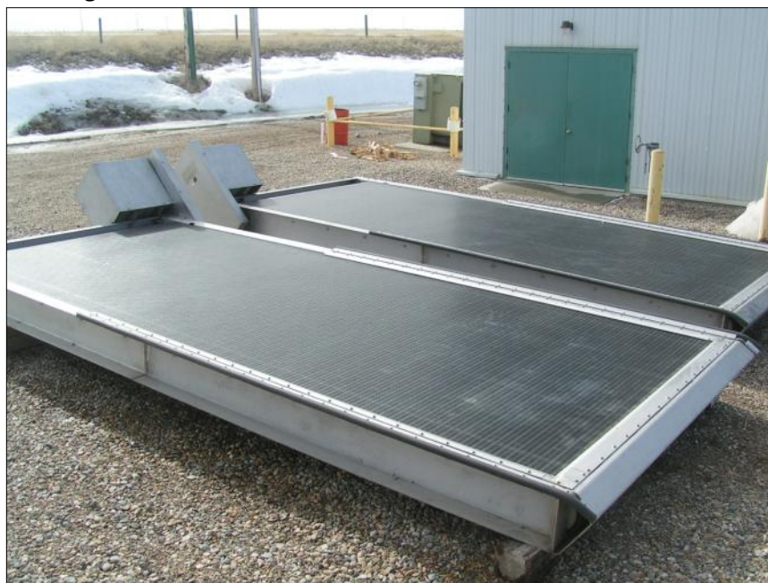
Travelling water screens to be installed
